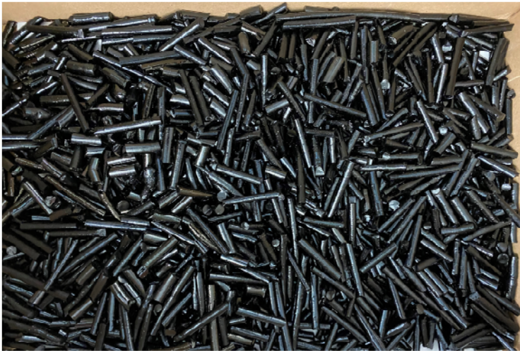
Pelleted asphalt binder from Solideum process ready for rail or truck transport
