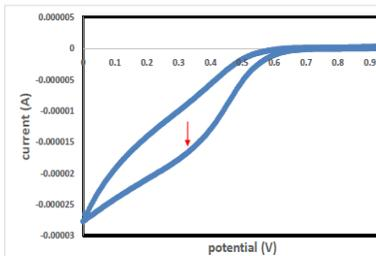
Figure 1 Cyclic voltammogram on a commercially available glassy carbon electrode in 1 mM Cr(VI)
