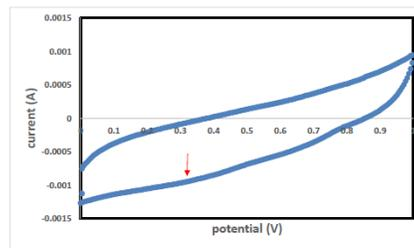
Figure 2 Cyclic voltammogram on lignochar coated carbon foil electrode in 1 mM Cr(VI) at pH 3.
