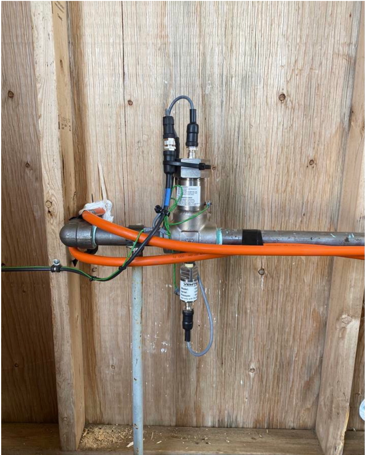
Figure 4. Ventsentinel® unit, field trails, close-up on the unit attachment to line.
