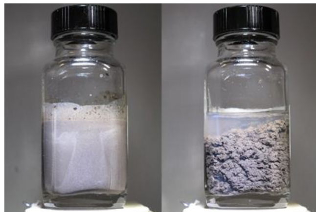
Left: Untreated mature fine tailings (MFT) with 30 wt% solid concentration. Right: MFT treated with InnoTech flocculant.
