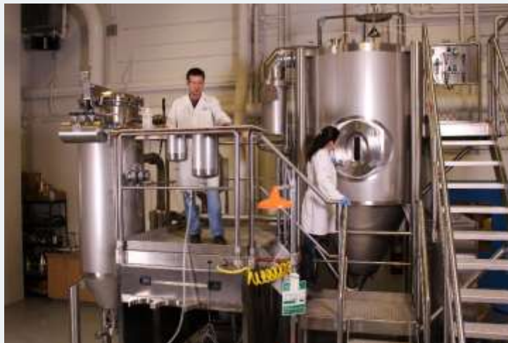
The dryer unit at InnoTech Alberta's CNC pilot plant removes moisture from the cellulose biomaterial.
