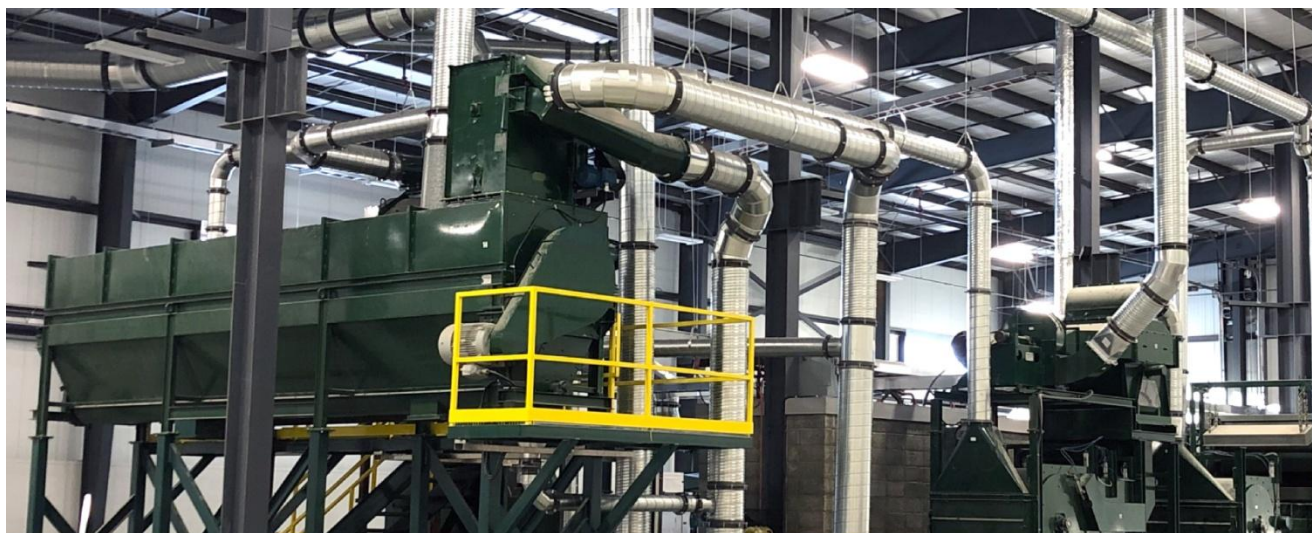
Natural Fibre Technologies' commercial hemp decortication plant in Nisku, AB separates hemp stalk into fibre and hurd.
