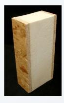
ABF-funded researchers are finding new ways to use oriented strandboard panels. Structural insulated panels (SIP) use OSB to encase rigid foam from canola that is strengthened with cellulose nanocrystals to create a wall system that does not need studs or a vapour barrier.
