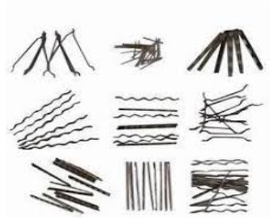
Different shapes of commercially available steel fiber. Steel fiber is dispersed at between 0.3% and 2.5% by volume in plain concrete.
