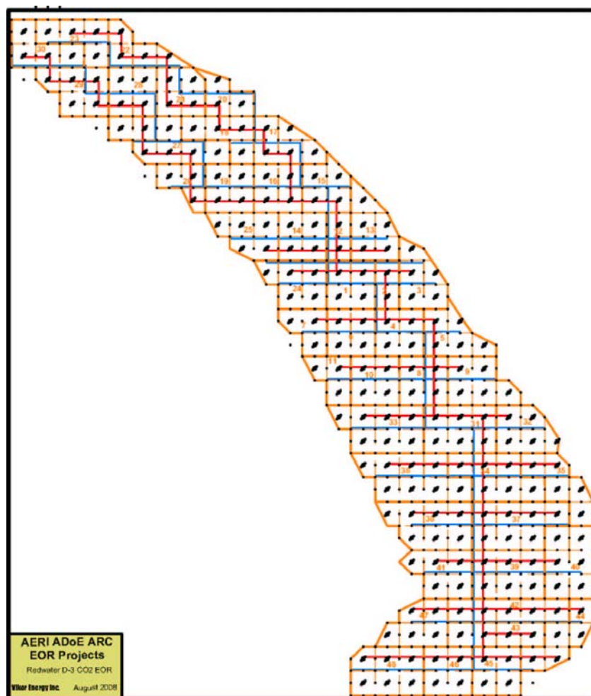
Figure 5.2.5.3: Pipeline layout showing new gathering system (blue) and water lines (red)
