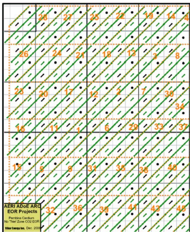
Figure 5.2.2.2: Pembina Cardium without thief zone - existing wells in black and new horizontal production wells (green lines) and new vertical injectors in green for a portion of Area 1.
