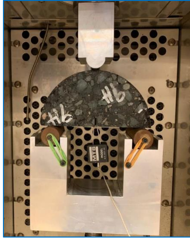
Figure 19. Semicircular bending (SCB) test with crack mouth opening displacement (CMOD) gauge.
