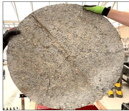
b) Carbon fiber reinforced samples exhibiting significant post cracking behavior
