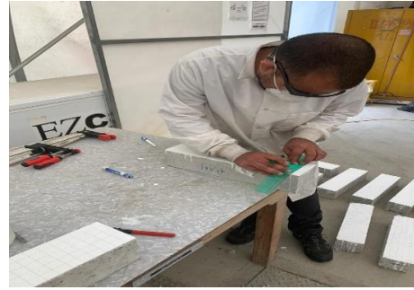
b) Preparation of Beam samples for testing
