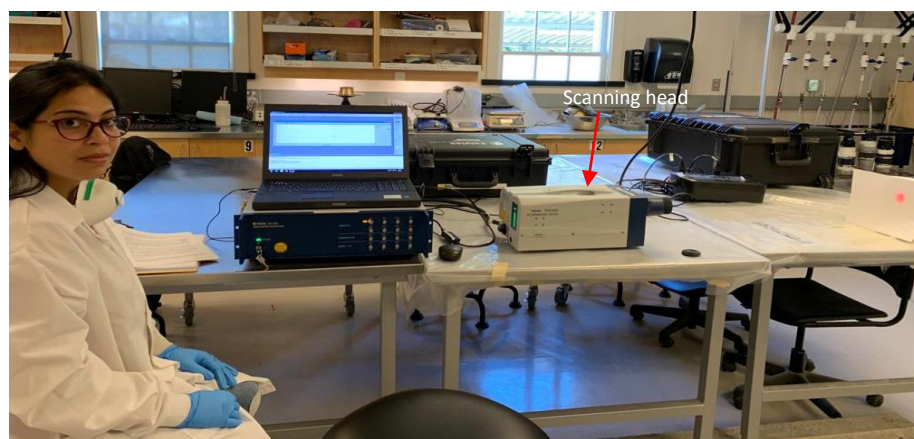
Fig. 4-2 Setting up Laser Scanning Vibrometer for evaluating Fiber reinforced concrete
