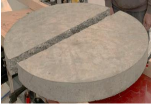
a) Control samples exhibiting a brittle failure and zero post crack strength
