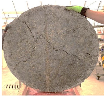
c) Triangular cracking in carbon fiber reinforced concrete
