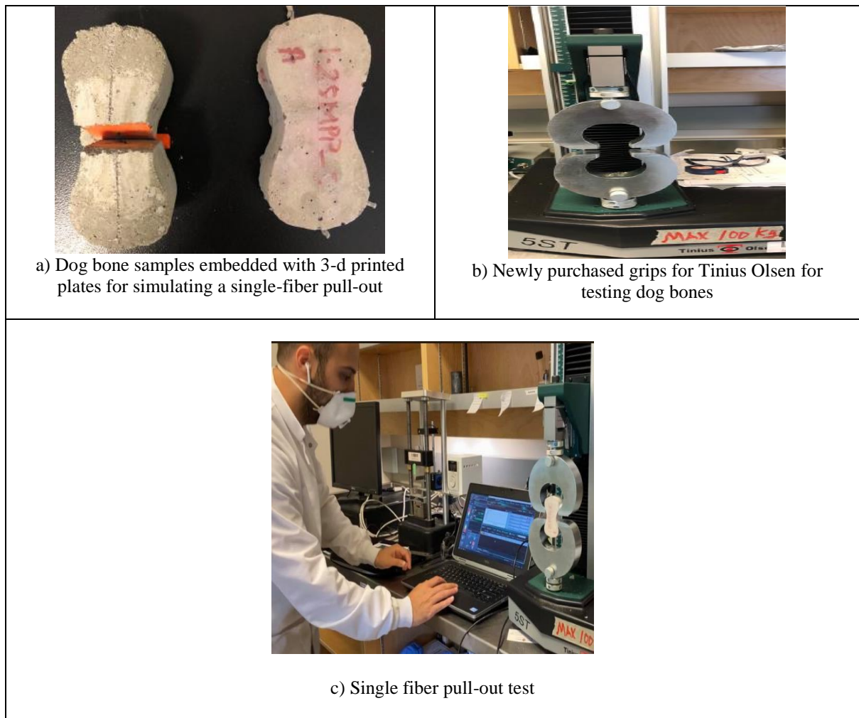
Fig. 4-1 Dog bone test for single fiber pull-out using Tinius Olsen
