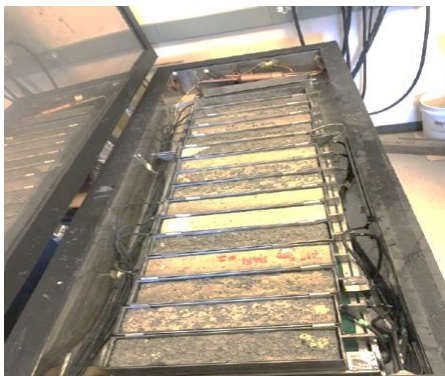
a) Carbon fiber reinforced concrete samples kept in Freeze thaw chamber
