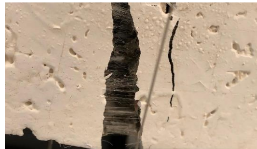
d) Stitching action of fibers
