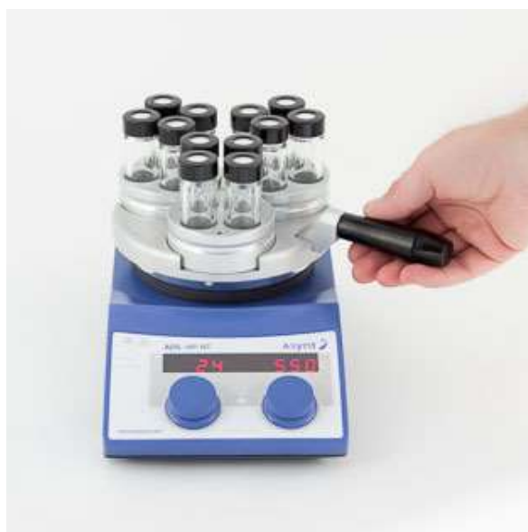
Figure 2 – Hot Plate Stirrer with multi-welled heating blocks
