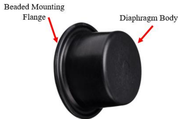
Figure 19: An example image of a rolling diaphragm. These types of devices are used to create a frictionless seal between the piston cylinder and piston. Different sizes are used for each of the different configurations
