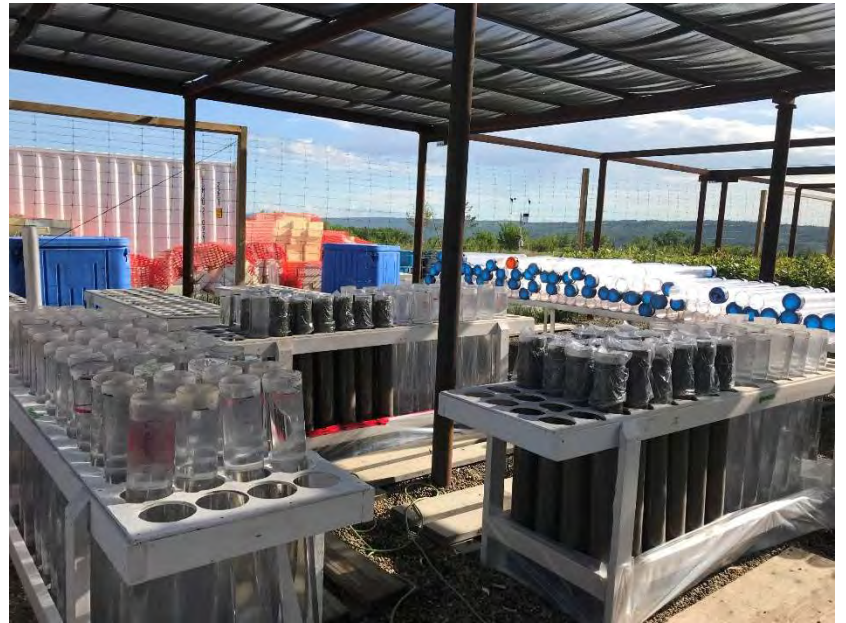
Figure D27. Photos of column establishment in June, 2018 depicting centrifuge cake in basin, filled columns, and members of the setup team preparing to homogenize tailings with mixer and drill
