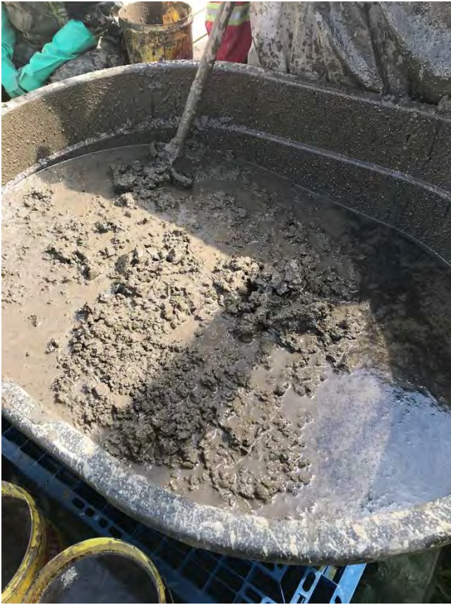
Figure D27. Photos of column establishment in June, 2018 depicting centrifuge cake in basin, filled columns, and members of the setup team preparing to homogenize tailings with mixer and drill
