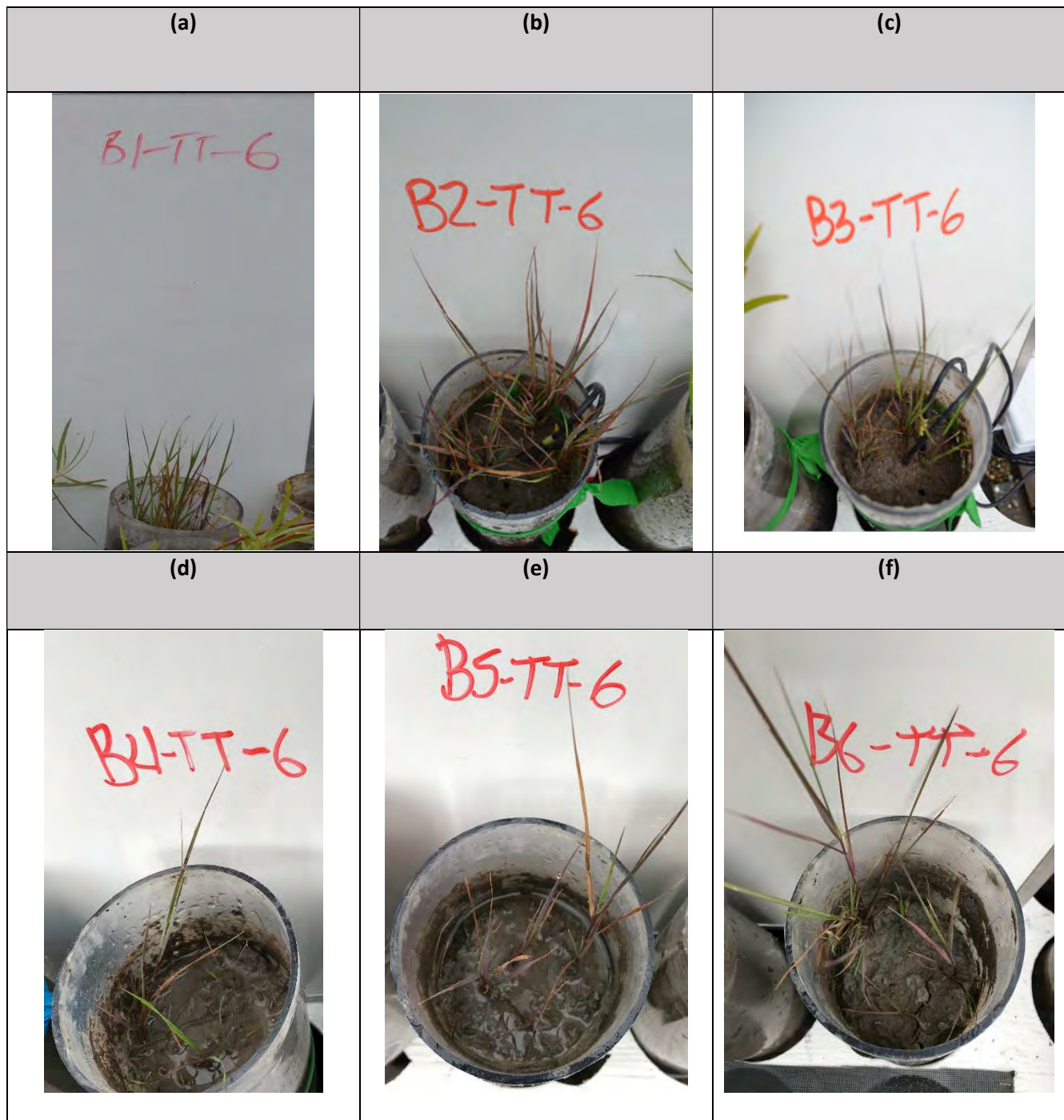
Figure D13. Photos of Elymus trachycaulus vegetation columns grown in thickened tailings without amendment (a-f) from September 6, 2018
