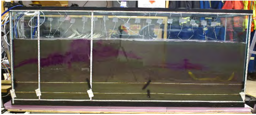
Figure 20 CFFT Filled the Tank to a height of 60 to 61 cm, Ready for Capping
