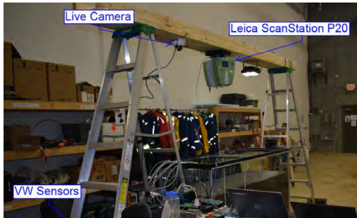
Figure 17 Leica P20 Scanner and Vivotek Camera Installation
