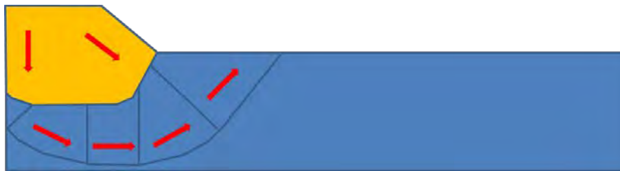
Figure 40 Sand Cap Penetrating Deep into the Tailings
