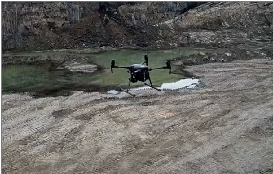
Figure 1 UAS survey of active mine face using a DJI M210.
