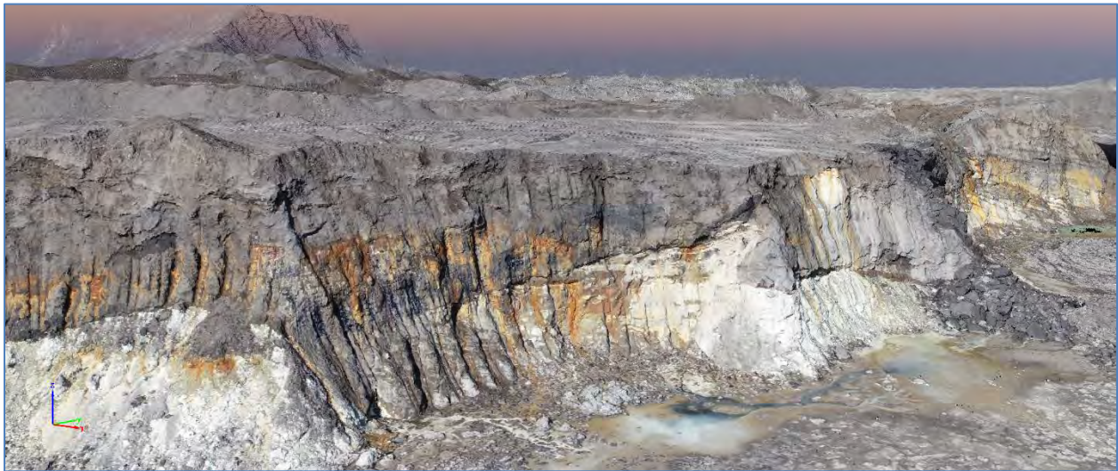
Figure 2 Example 3D model generated for an active mine face.
