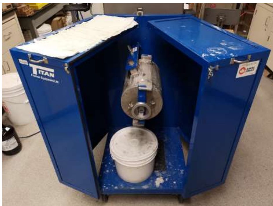
Figure 2 Rod mill from Titan Process Equipment Ltd.
