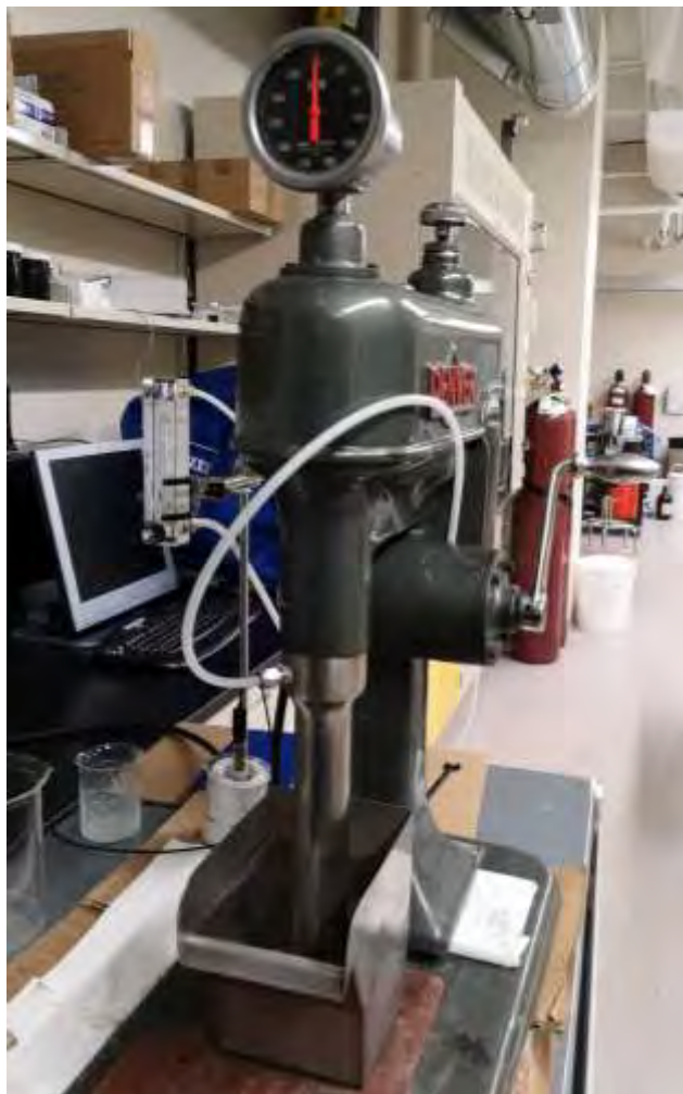
Figure 3 Denver D-12 flotation machine.
