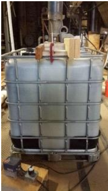
Figure 5. Image of 1 cubic meter tote used to store and mix tailings material (surrogate test).
