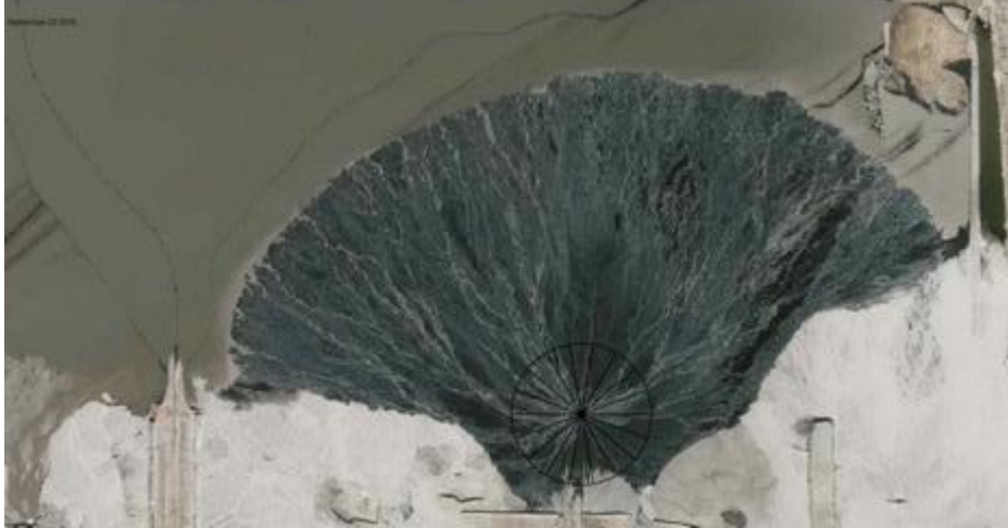
Figure 1. Aerial image taken over a TSRU tailings beach formed in an external tailings facility.
