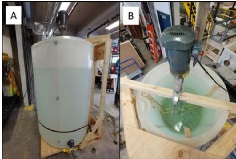
Figure 33. Images of the mixing tank used for TSRU tailings experiments. A large variable speed mixer with long shaft was added. Internal baffles were installed on the perimeter of the tank as well.
