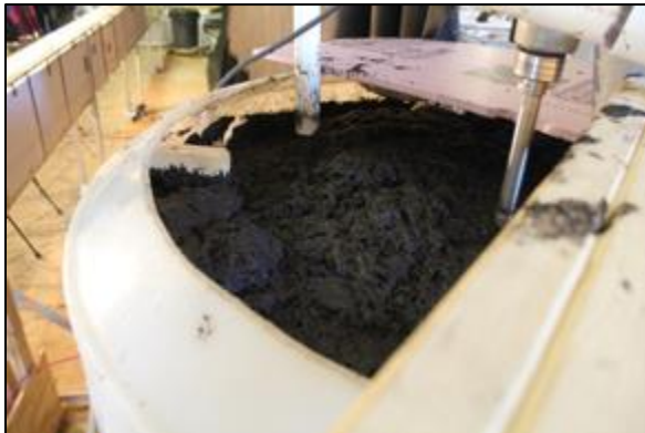
Figure 34. Image of mixing vessel prior to a TSRU experiment. Pink insulation was used to cover the tank and was slid to the side in order to collect samples from the tank.
