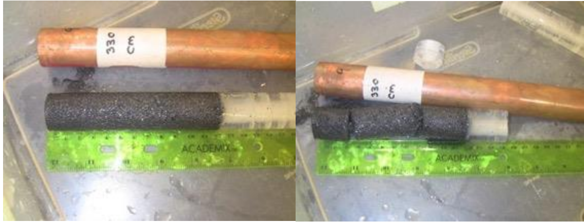
Figure B2. Images of extruded, frozen core (left) and sectioned into bottom, middle and top (right).
