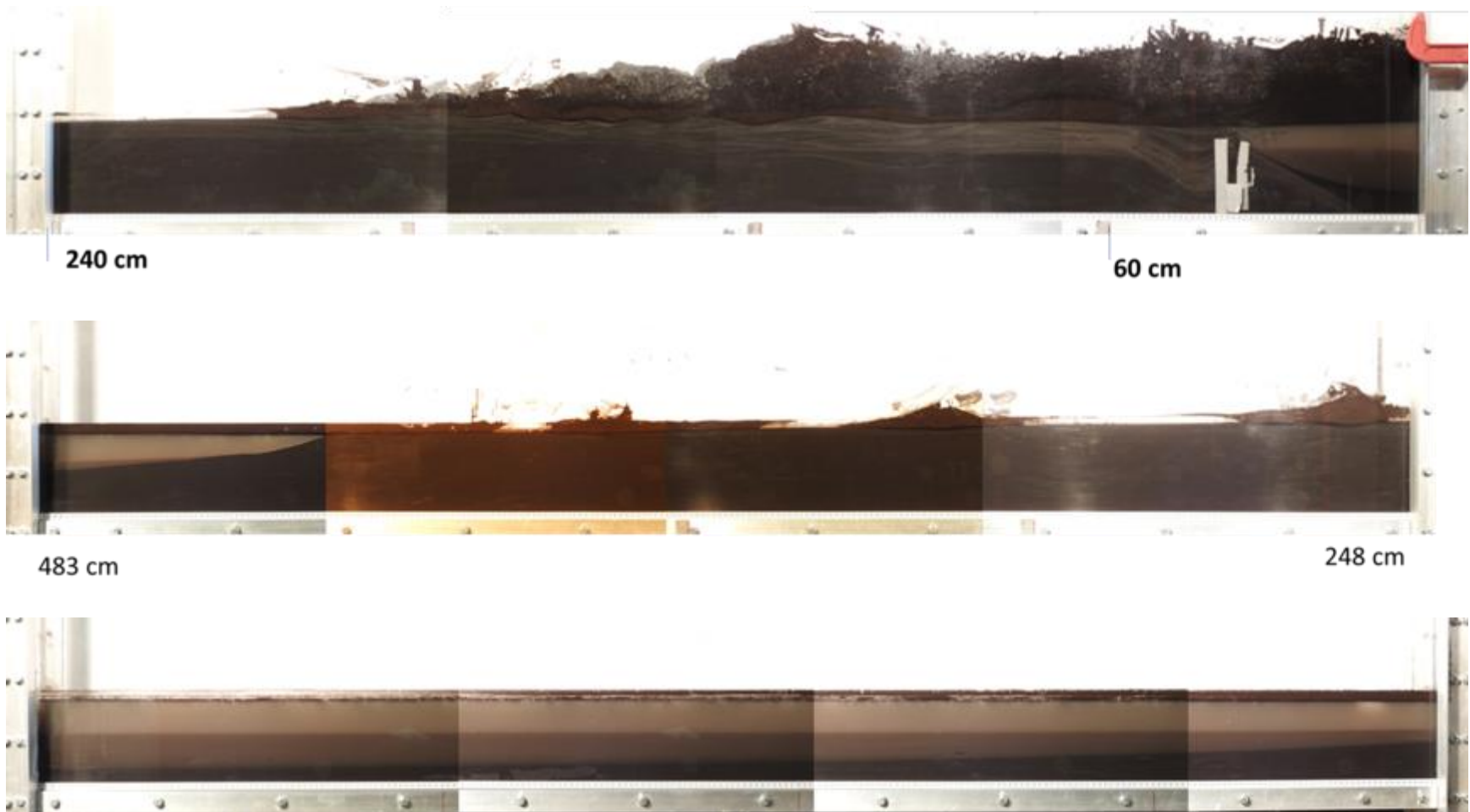
Figure 41. Composite images taken of the final deposit of T_02 (input discharge = 0.25 l/s). Flow was from right to left.
