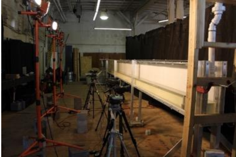
Figure 10. Image of the flume setup showing video cameras and lighting immediately prior to the start of a TSRU tailings experiment.
