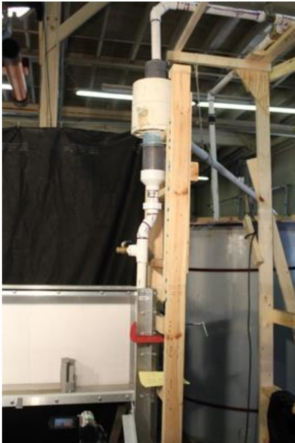
Figure 36. Image of mixing tank (background), recirculation plumbing and constant head tank leading tailings slurry into research flume.
