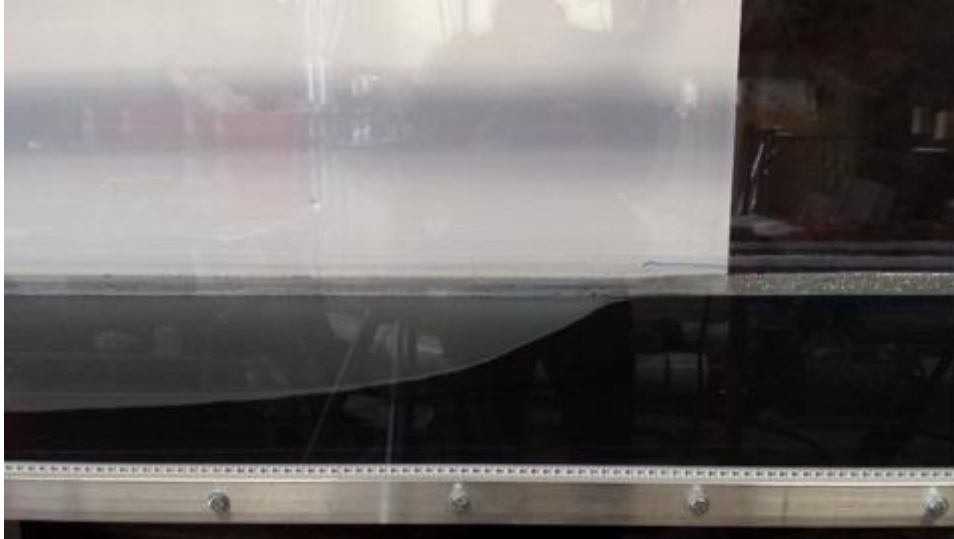
Figure 28. Image taken of the final deposit several hours after the end of Surrogate Test 3. The water surface is at the end of the beach. A fine grained solids layer (grey) can be seen draping the bottom set deposit resulting from suspension settling.
