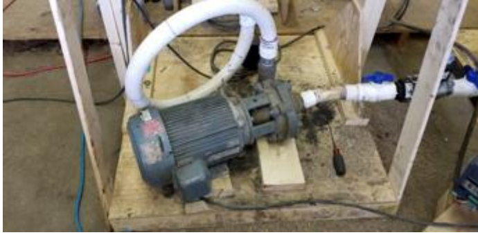
Figure 35. Image of the centrifugal pump used to deliver TSRU tailings to the research flume.
