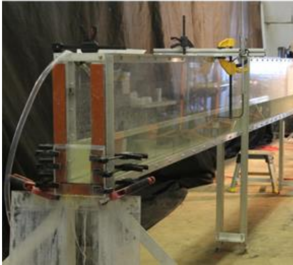
Figure 9. Image of end plate on flume that was used to establish a 15-cm water depth in the flume. The end-plate also had a beveled top edge and served as a sharp-crested weir for discharge measurements. A manually operated point gauge was used to measure water surface prior to and during an experiment.
