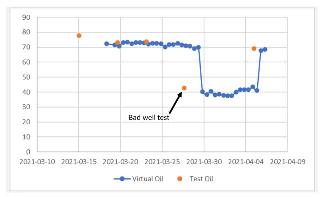
If the VFM had kept running based on the consistent well test from March 23rd, the VFM trend would have remained consistent also. In the event of a bad test, it is likely that the VFM can continue to provide good flow estimates if the most recent consistent well test is used.
