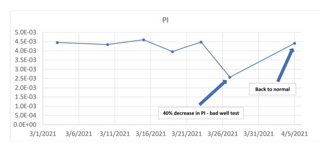
The chart below shows the performance of the same set of well test calibrations with the VFM in March 2021.
