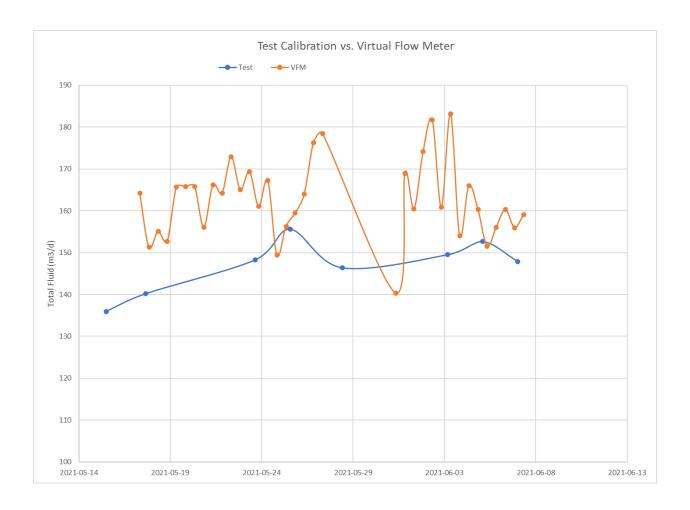
On investigation, the VFM runs were consistently underestimating FBHP against the manual measurement, shown below. A lower FBHP means higher rates.
