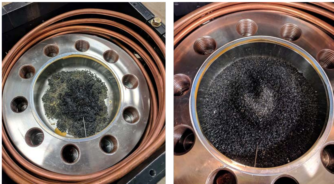
Figure 9: Picture of showing the reactor content after reaction. Left – Stearic acid was used as feedstock with SiC as heating aid; Right – Oleic acid was used as feedstock with SIC as heating aid on the 2.45GHz system. Evidence of hotspot can be seen as the scotched areas near the centre of the SiC.
