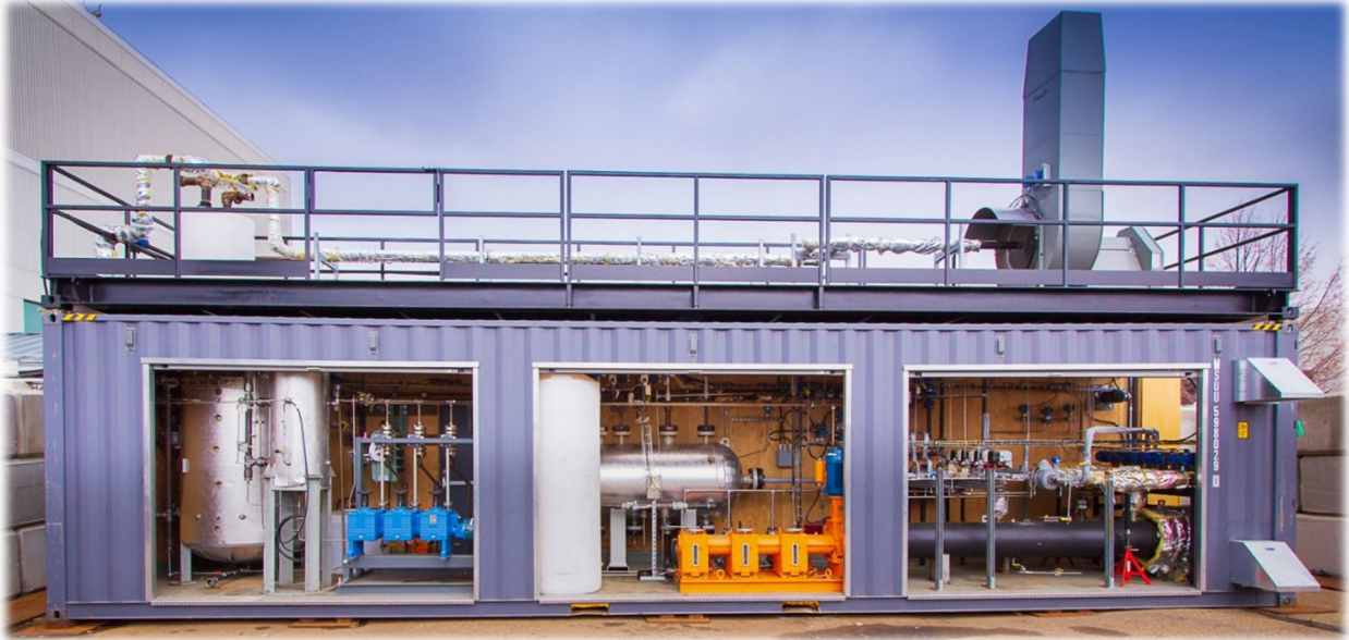
Figure 4.1 Completed ICD & Solvents Flow Loop
