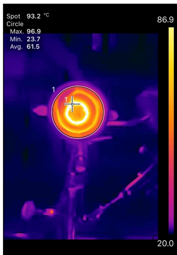
Figure 2. The measurement of reactor temperature by infrared camera after reaction
