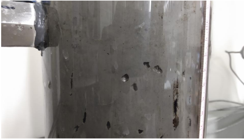
Figure 4.31. Photographs of amended column during incubation: Pores in tailings created by biogases – methane and carbon dioxide- during active methanogenesis
