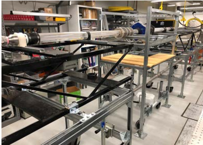
Figure 31 Pipe frame and section with FRM and optical tomography system.
