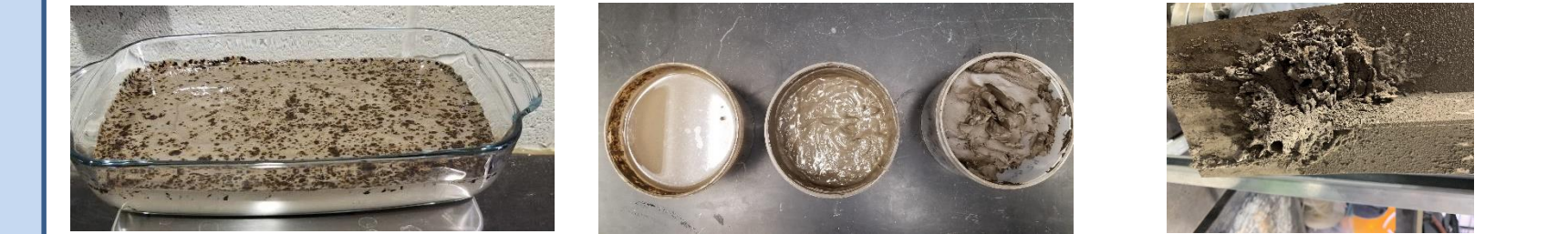
MFT "as received" at 25% Solid: 25%, 50%, 70% Solids on impact plate
