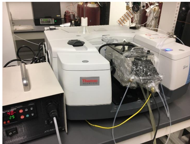
FTIR with in-situ chamber and gas cell
