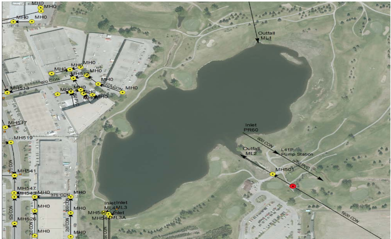
Figure 1. Aerial photo of McCall Lake. The yellow circles represent storm manholes, the orange squares represent catch basins, the black arrows indicate the direction which storm drains flow, and the black lines are storm pipes [provided by The City of Calgary].
