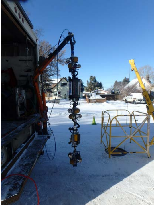
ACPS robot prior deployment (left) and being inserted into manhole (right).
