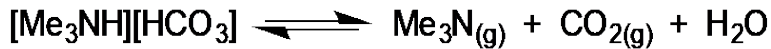
Figure 1. “Switchable” formation and decomposition of trimethylammonium bicarbonate. The salt formed on the left side of the equation acts as the forward osmosis draw solute
