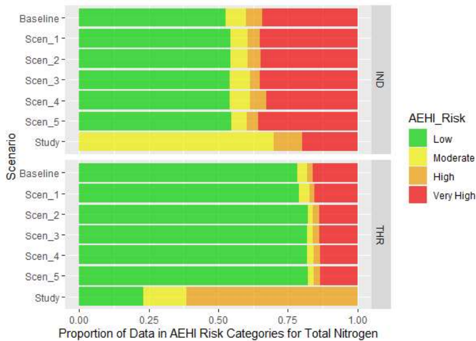
Figure 4-13. Proportion of monthly flow-weighted mean concentrations of total nitrogen (TN) falling within the aquatic ecosystem health impairment (AEHI) risk categories derived for Indianfarm (IND) and Threehills (THR) creeks. Scenarios refer to the CEEOT simulation scenarios and the Study refers to the number of samples collected during the 2016 – 2018 field sampling matched against the AEHI risk categories.
