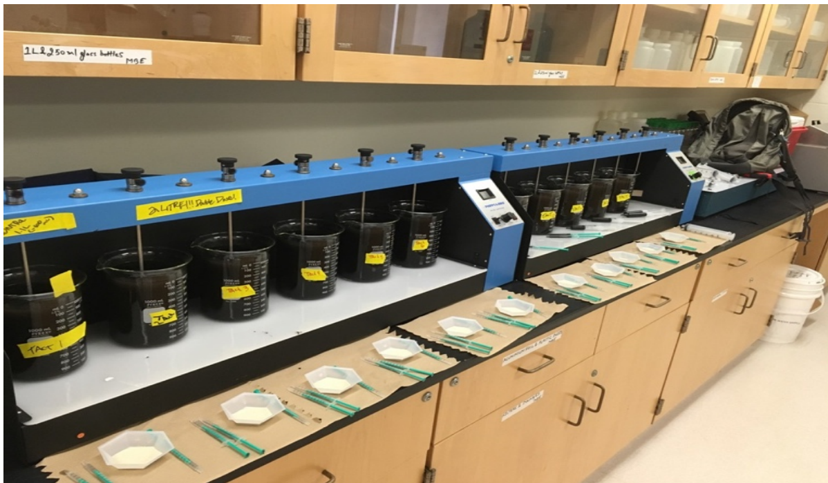
Figure 23. Jar testing of BSF with a rise rate of 40 m/hr and sand dose of 10 mg/L. A polymer dose 0.5 mg/L was used throughout the tests.
