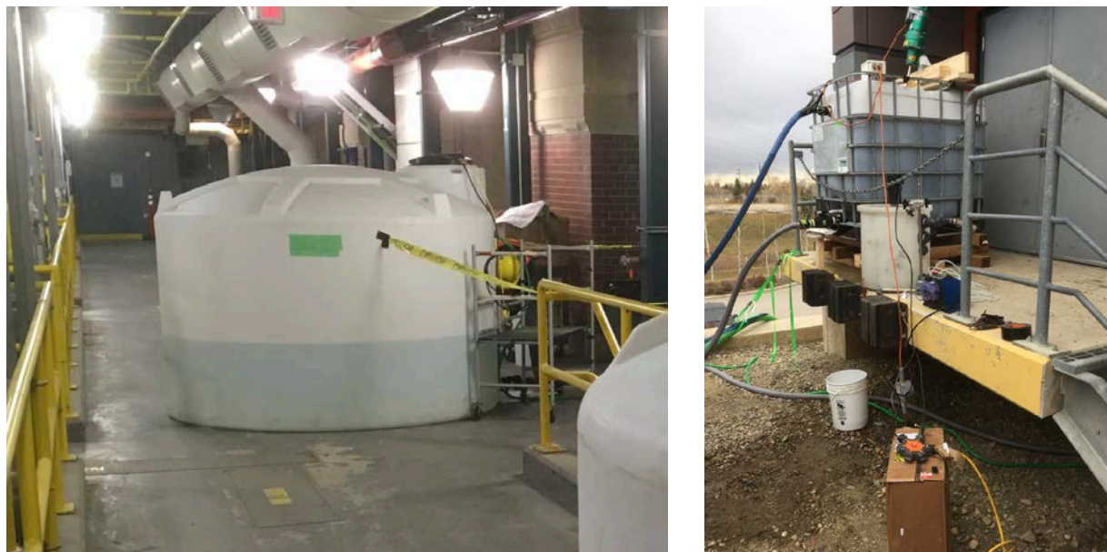
Figure 28. Raw water storage tank (5,000L capacity) used to prepare severely deteriorated “black-water” matrices using during pilot-scale BSF investigations (left) and raw water storage tank during pilot-scale BSF investigation (right).
