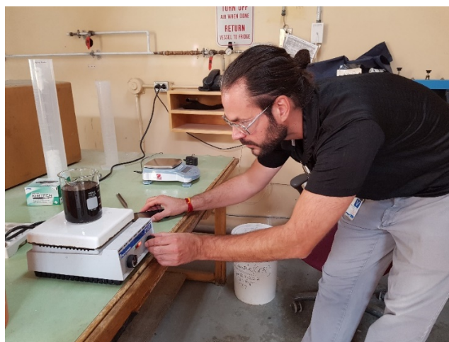
Figure 21. Generation of simulated severely deteriorated (“black-water”) water matrices representative of “worst-case scenario” conditions after severe wildfire.
