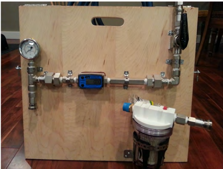
Figure 1: Water sampling device (WSD) created for the project and used for collecting a large volume of well water for enteric virus testing.
