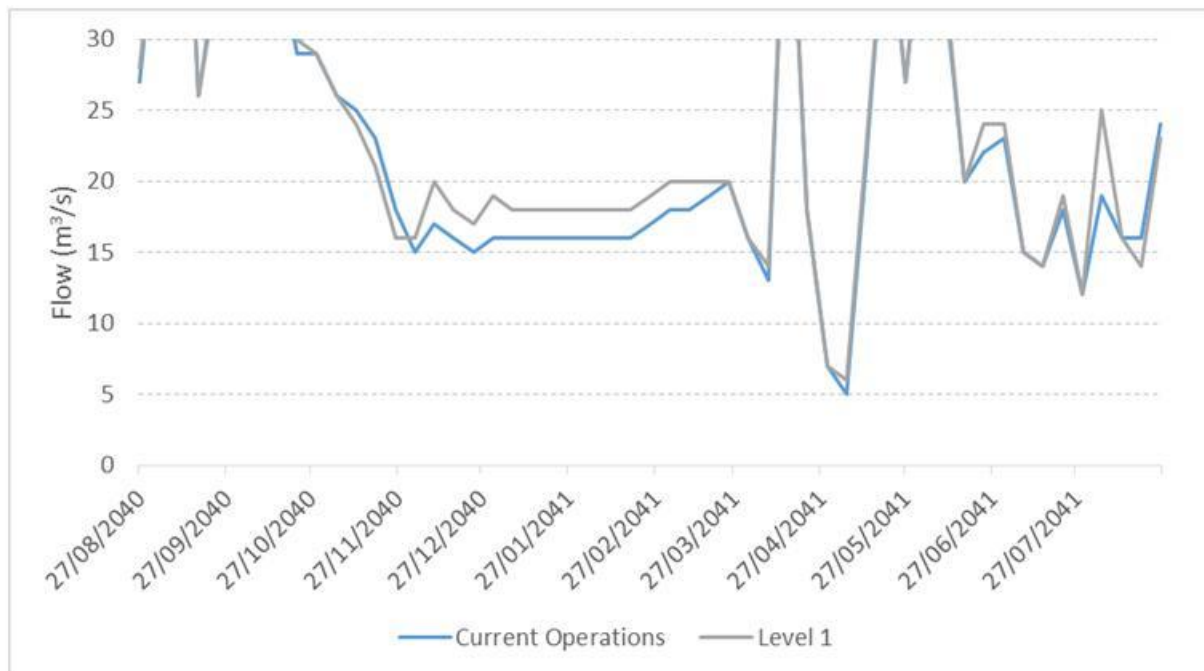
Figure 28: A comparison of streamflow (m 3 /s) in the Red Deer River at the mouth of the Red Deer during current operations (blue) and operations that aim to address downstream needs (grey)
