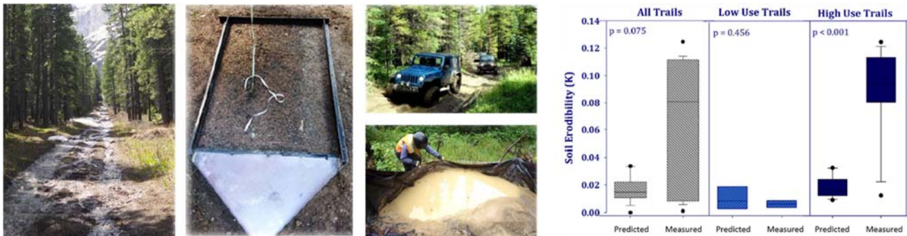
Figure 23 – Comparison of measured and predicted erodibility for high and low use intensity trails
