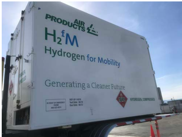
Photo: Example of an Air Products portable gaseous supply product. The Air Products Liquid to Gaseous Portable Hydrogen Fueler will combine both liquid storage and gaseous dispensing systems.
