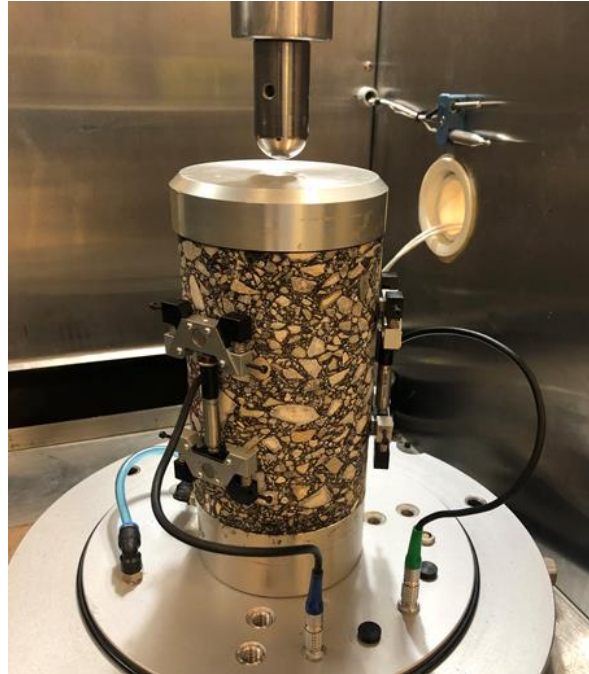
Figure 12. Dynamic modulus test set up with LVDTs
