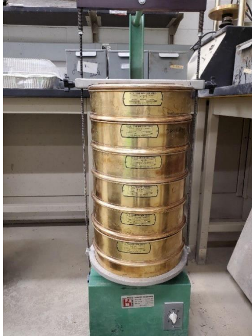
Figure 21. Sieving device with different sieve sizes
