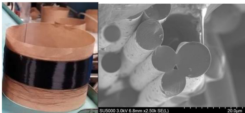
Figure 1. (a) Melt-spun asphaltene fibers produced from as-received sample A (also called S1); and (b) Asphaltene fibers stuck together during oxidative stabilization.
