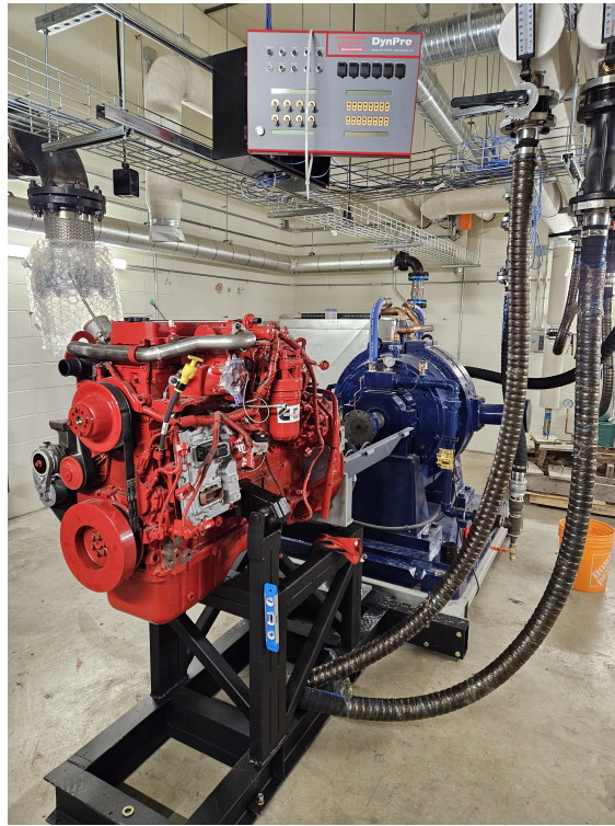
Figure 1: Engine Testcell - Engine and Dynamometer
