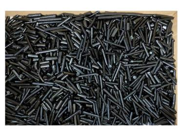
Pelleted asphalt binder from Solideum process ready for rail or truck transport.
