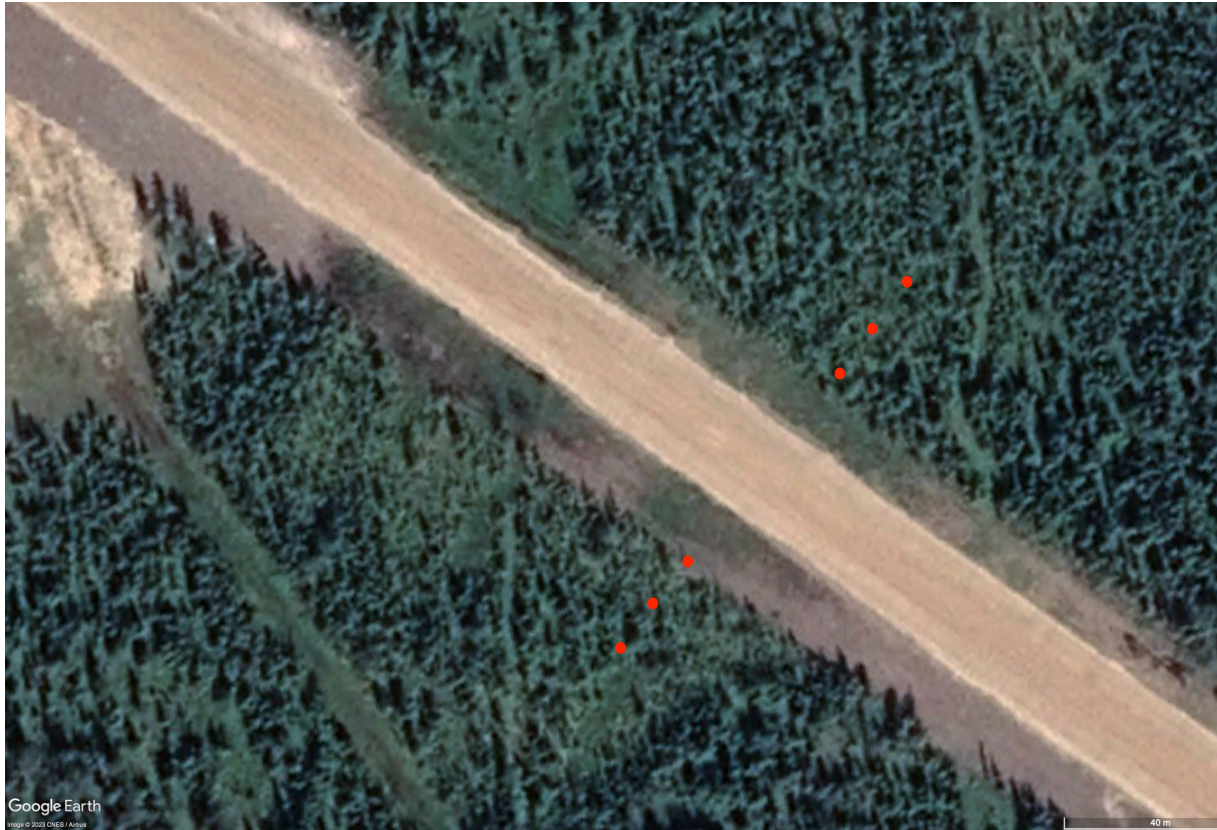
Figure 6. Example of water well placement in original transects established in 2018. Wells were placed 15, 30, and 45 m from each edge of the road. Water flow is from southwest to northeast. Image is of Transect 3 area shown in Figure 5 above.
