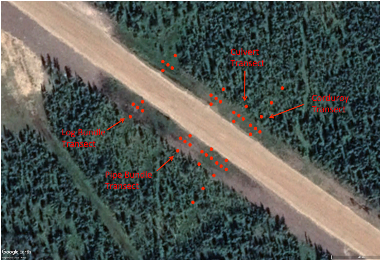
Figure 7. Layout of well and piezometer transects for conduit performance assessment. Wells were placed at 1, 5, and 15 m from each edge of the road immediately in front of a culvert, log bundle, and pipe bundle. Piezometers were installed approximately 1 m on either side of the well at 5 m from road edge. The southeast-most transect incorporated the original well transect established in 2018 and was situated between a pipe bundle and culvert.
