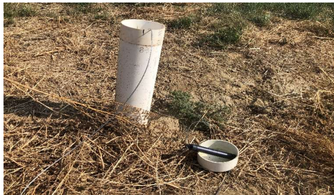
Figure 3. Sampling well with pressure transducer removed and resting on cap awaiting downloading.
