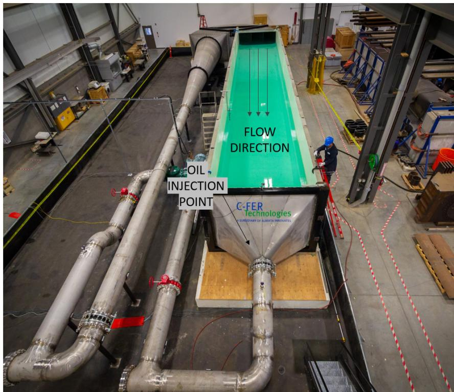
*Figure 2 Oil Injection Point in IWS*
