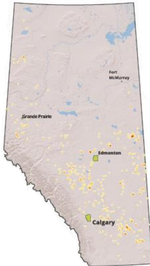
Figure 9. Heatmap showing the distribution of methane emissions from surface casing vent flows reported in 2021. Map developed by MWA, data from AER (Alberta Energy Regulator, 2023a).
