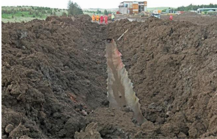
Figure 1: Result of a Full-Scale Test to Verify Fracture Propagation Arrest Capabilities for a Dense-Phase CO 2 Pipeline
