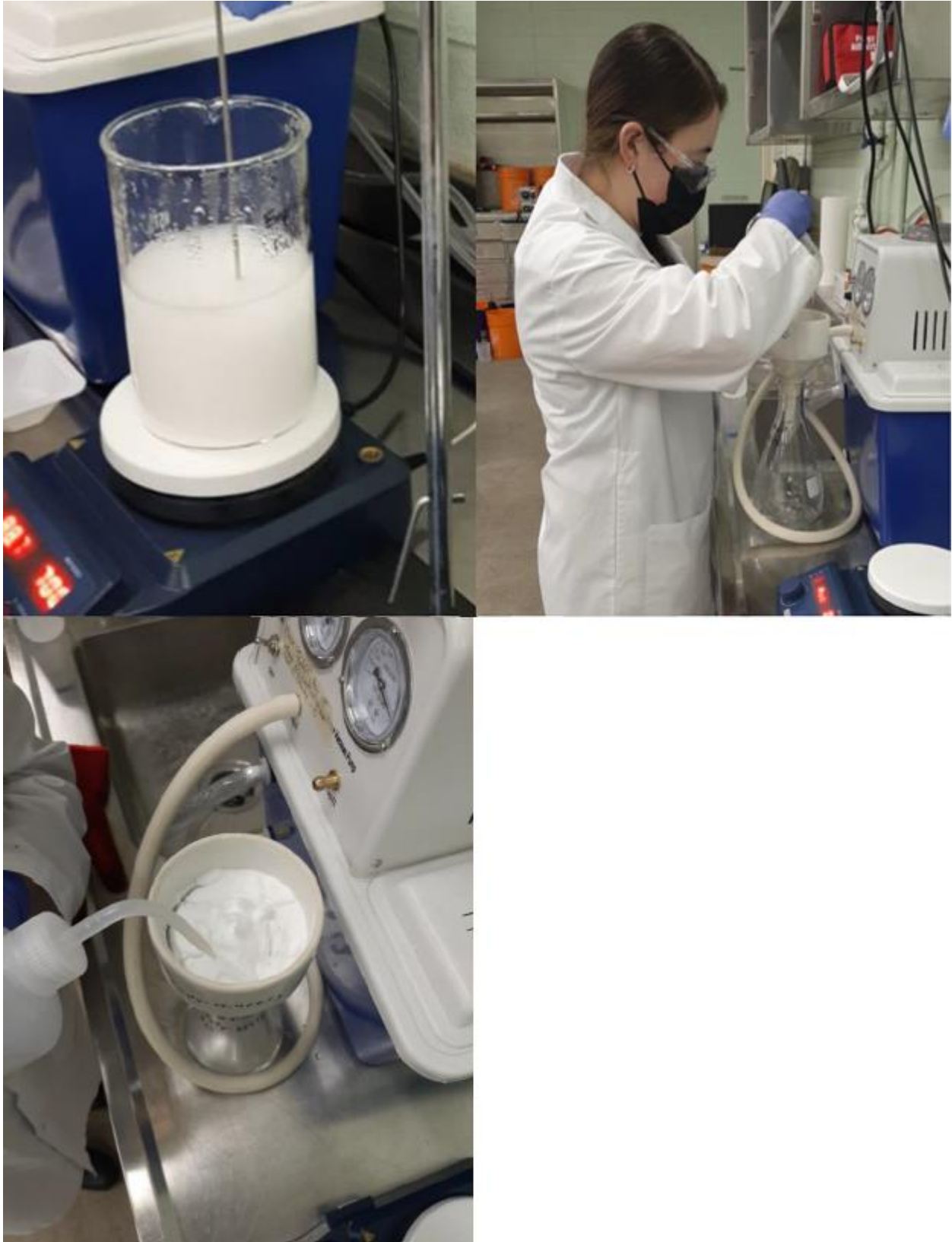
Figure 6: (Top Left) Precipitate Formation, (Top Right) Filtration, and (Bottom Left) Filter Cake Washing
