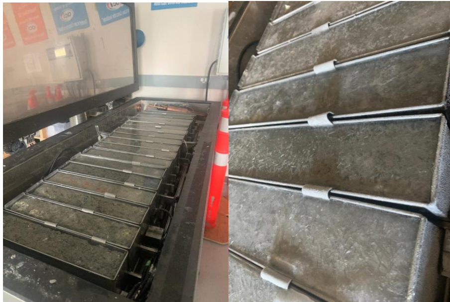
Fig. 19. Freeze-thaw test on beams
