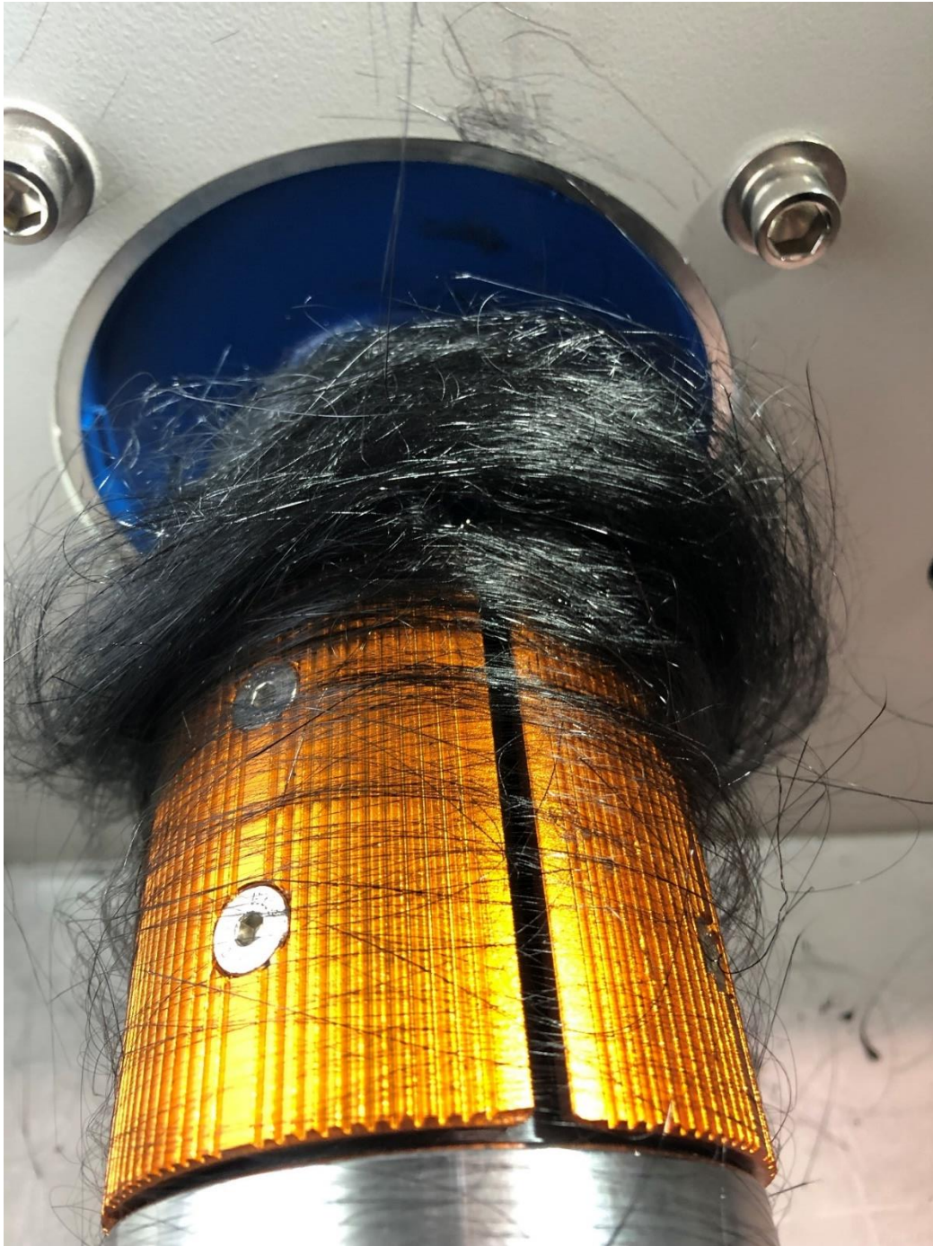
Green fibre output from the melt spinner – yielding filaments in excess of one meter long.
