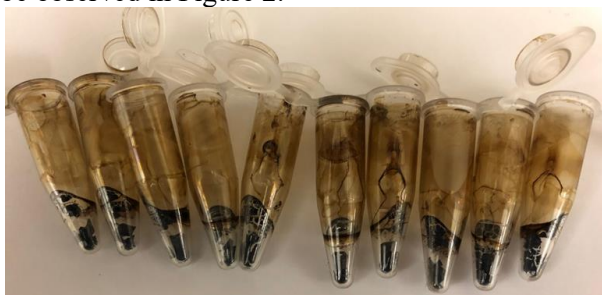
Figure 2. Insoluble residuals found in asphaltene after the cleaning process
