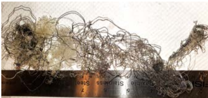
Figure B2. Filaments obtained from the spinning trial 2 with non-uniform distribution of Asp/PS (brown regions) in PAN (white/yellow regions).
