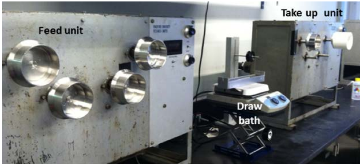
Figure 3. Experimental set-up for hot drawing of the as-spun fibers. The as-spun fibers were mounted on the feed rollers, are then passed through the glycerol draw bath, and then finally collected on the take-up rollers.
