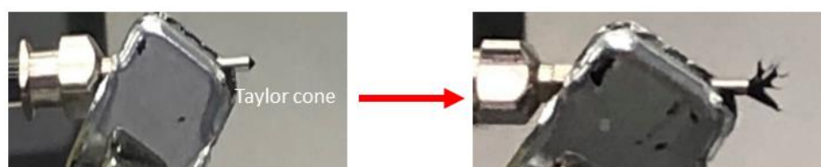
Figure 9 The clogging of the spinneret from normal Taylor cone to the dried sample clogging
